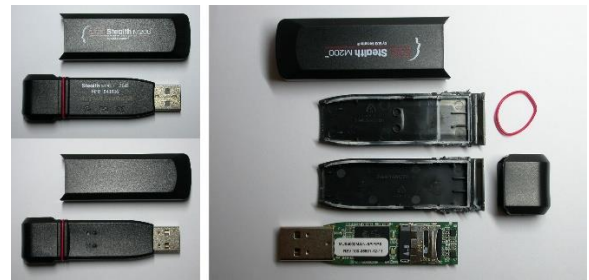
Fig. 48. Stealth M200 before and after opening its plastic case
