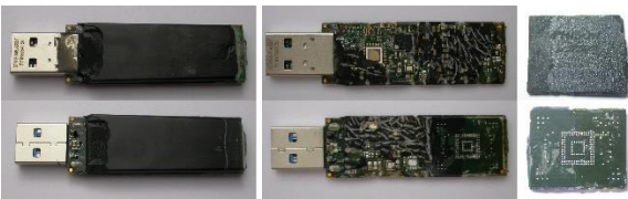
Fig. 22. IronKey S1000 before and after epoxy removal
