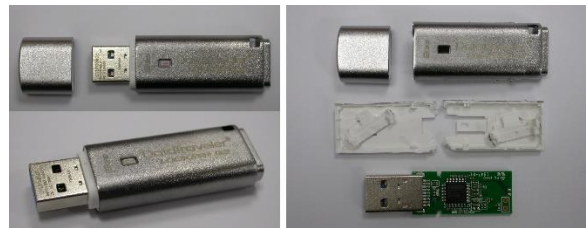
Fig. 32. DataTraveler Locker+G3 before and after opening its plastic case
