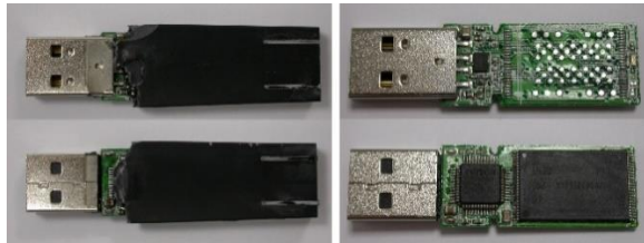
Fig. 3. IronKey device before and after epoxy removal
