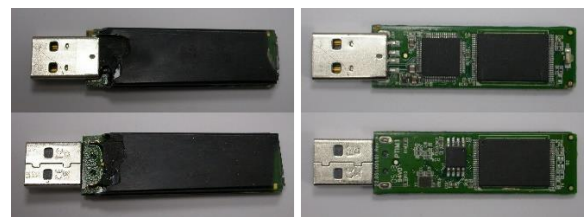
Fig. 17. IronKey D250 before and after epoxy removal
