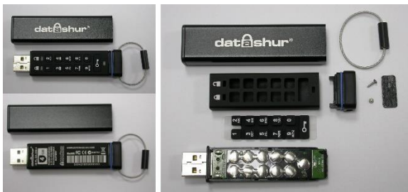
Fig. 46. Datashur before and after opening its metal case
