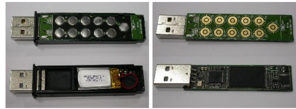
Fig. 47. Datashur before and after epoxy removal
