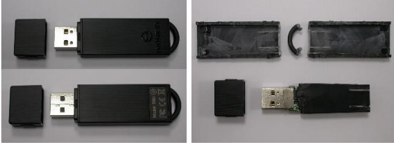
Fig. 19. IronKey D80 before and after opening its plastic case
