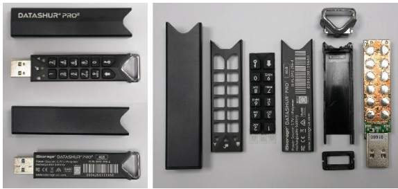
Fig. 43. Datashur Pro2 before and after opening its metal case
