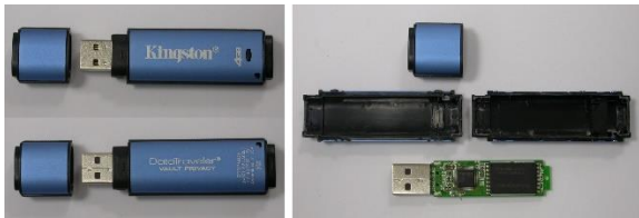
Fig. 36. DataTraveler Vault Privacy before and after opening its plastic case
