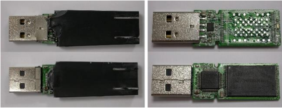
Fig. 20. IronKey D80 before and after epoxy removal
