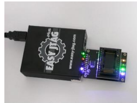
Fig. 62. Testing NAND Flash from IronKey D80
