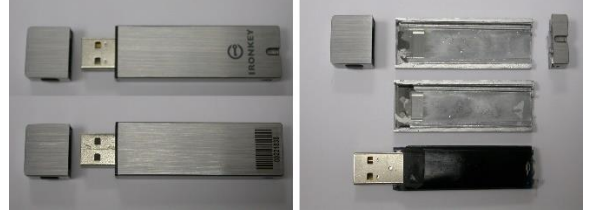
Fig. 8. IronKey D2 Ver.2 before and after opening its metal case
