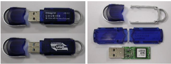
Fig. 52. Integral Courier before and after opening its plastic case
