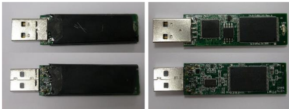
Fig. 12. IronKey S200 before and after epoxy removal
