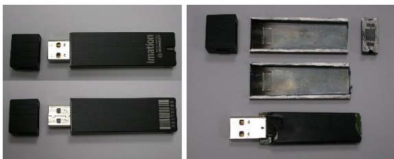
Fig. 1. IronKey device before and after opening its metal case
