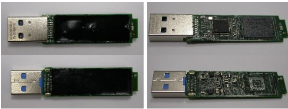
Fig. 28. DataTraveler DT4000G2 before and after epoxy removal
