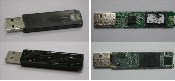
Fig. 5. IronKey D2 before and after epoxy removal
