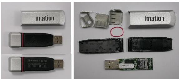
Fig. 14. IronKey F150 before and after opening its plastic case
