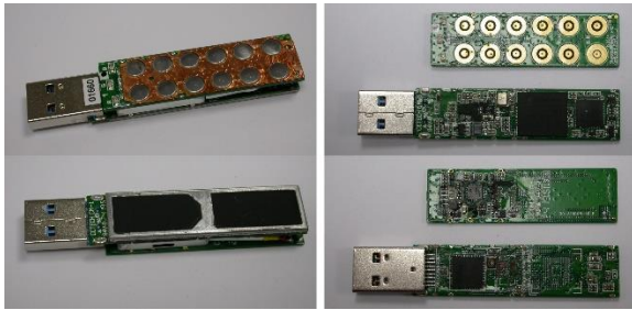
Fig. 44. Datashur Pro2 before and after epoxy removal
