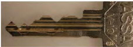
Figure 13.2: Key for a sidebar lock
